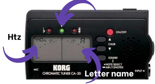
Low D string should be 147htzMiddle A string should be 220htzHigh D strings should be 294htz
